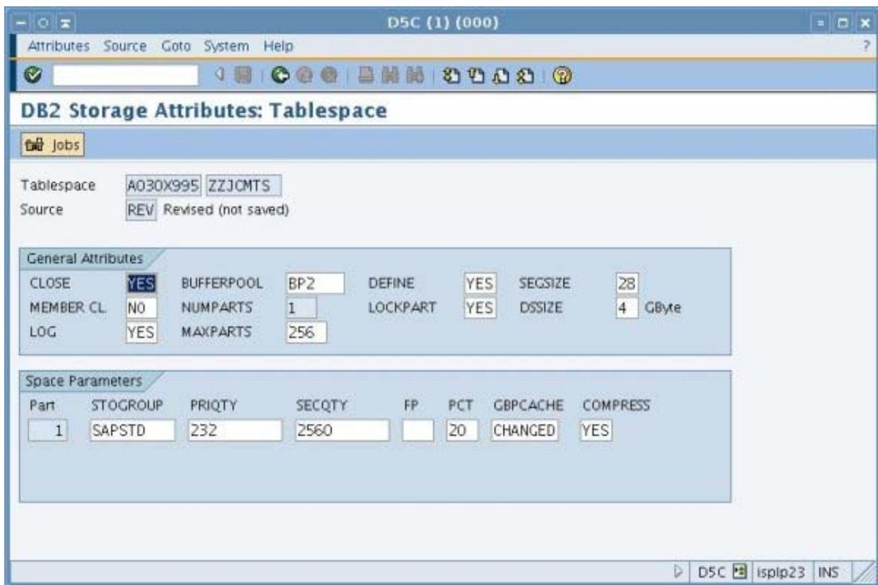
Figure 3-4 Define MAXPARTITIONS and DSSIZE parameter in SE14
