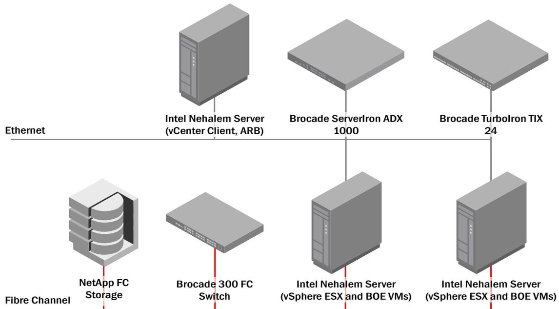
Figure 2 System Architecture
