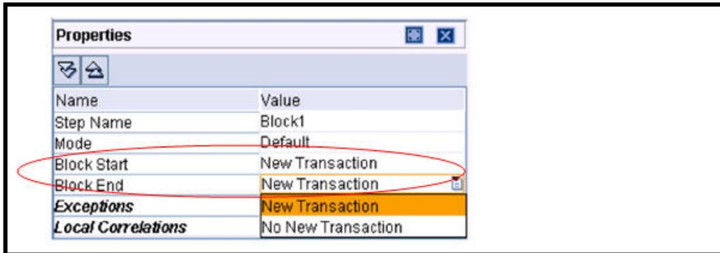
Picture 2: Configuration of a block start and end
