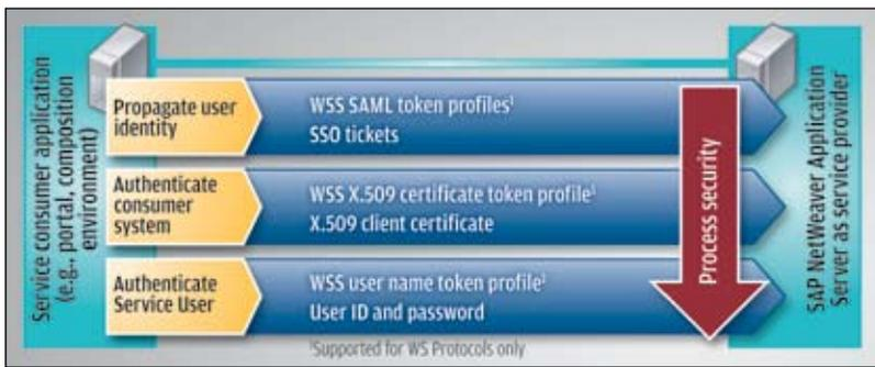
FIGURE 2 ▲ Authentication methods to support secure access to service applications
