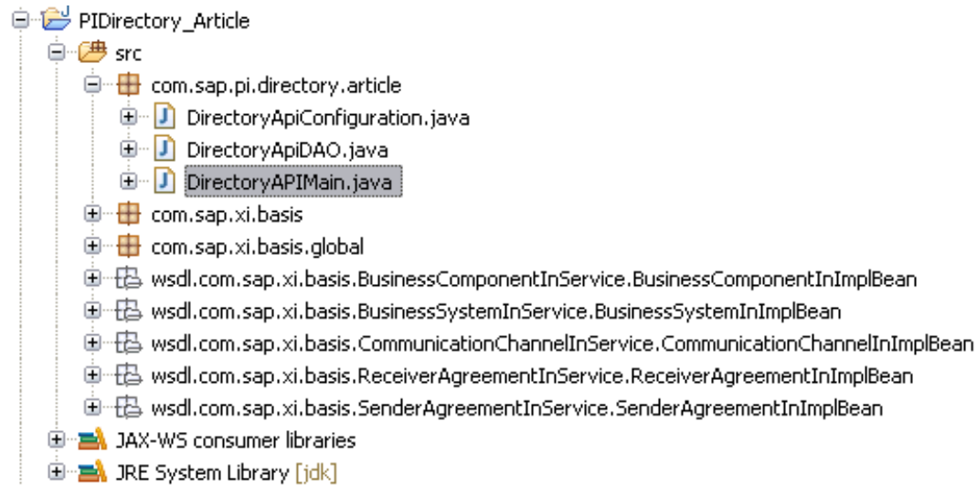
Figure 8: NWDS project structure showing manually created Java classes as well as generated web service clients
