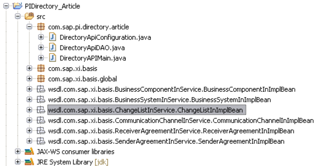
Figure 10: NWDS project structure showing the newly added web service client for change list support
