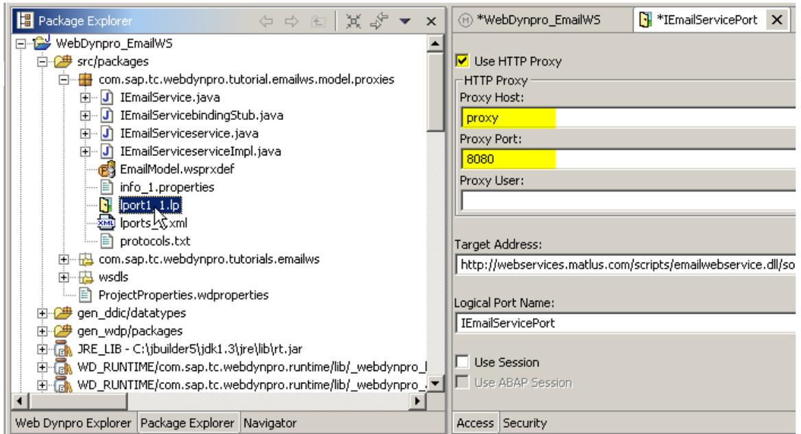
The field *Proxy Host* represents the host name or the IP address of the proxy server, and *Proxy Port* is the port to which the proxy server listens.
