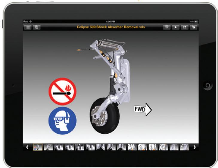
**FIGURE 3** ▲ Technicians can access visual maintenance instructions on a mobile device
