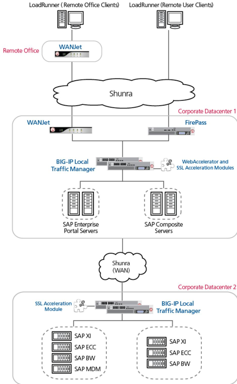
**Figure 4. Test landscape (Dotted lines represent physical servers, which each contain multiple application instances.) For High Availability and for scaling processing capacity application and network components of the same kind are doubled.**
