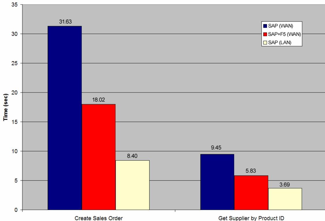
**Figure 8. Application Performance improvements with F5 and a 768 Kbps link**
