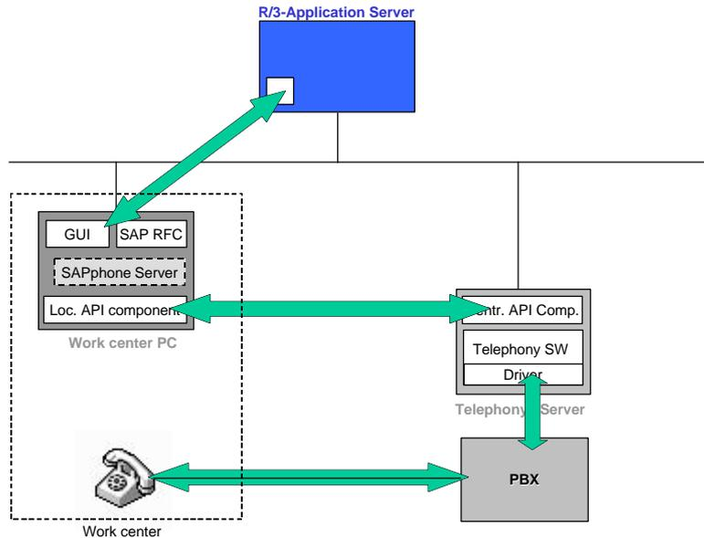
**Figure 4: Client/server solution with connection via network-capable API**
