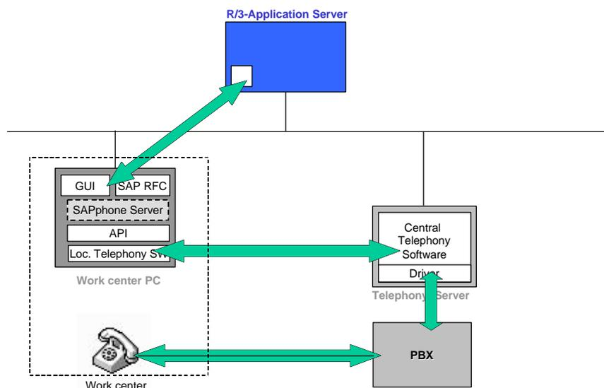
**Figure 3: Client/server solution with telephony software component on the work center PC**
