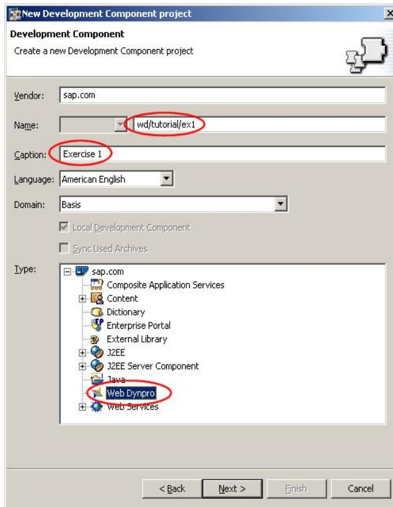
Figure 3: Create the Development Component of type Web Dynpro
