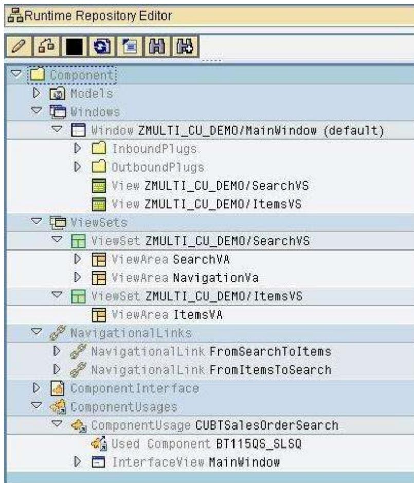
**Note:** Notice that only one component has been declared under component usage, the search component and nothing has been assigned to the view area of the ItemsVS page.
