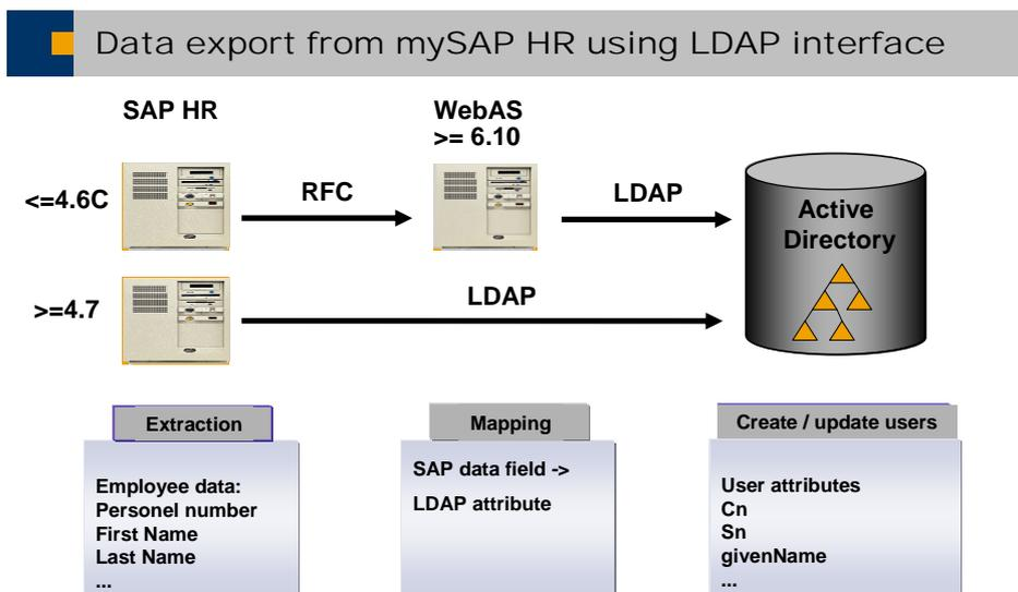
If SAP HR is running on a SAP Enterprise System or higher the function module `SPLDAP_RECEIVE_ATTRIBUTES` can be called locally.
