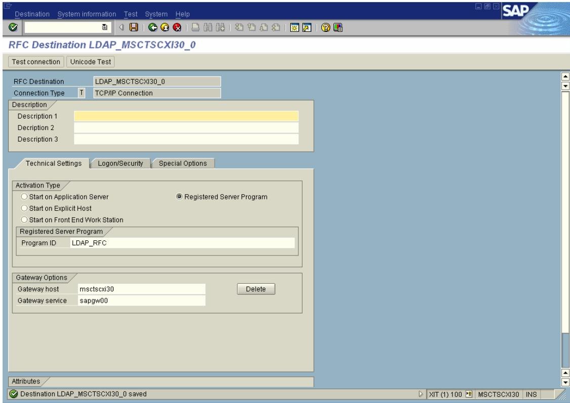
Figure 1: Configuration of the RFC destination of the LDAP Connector
