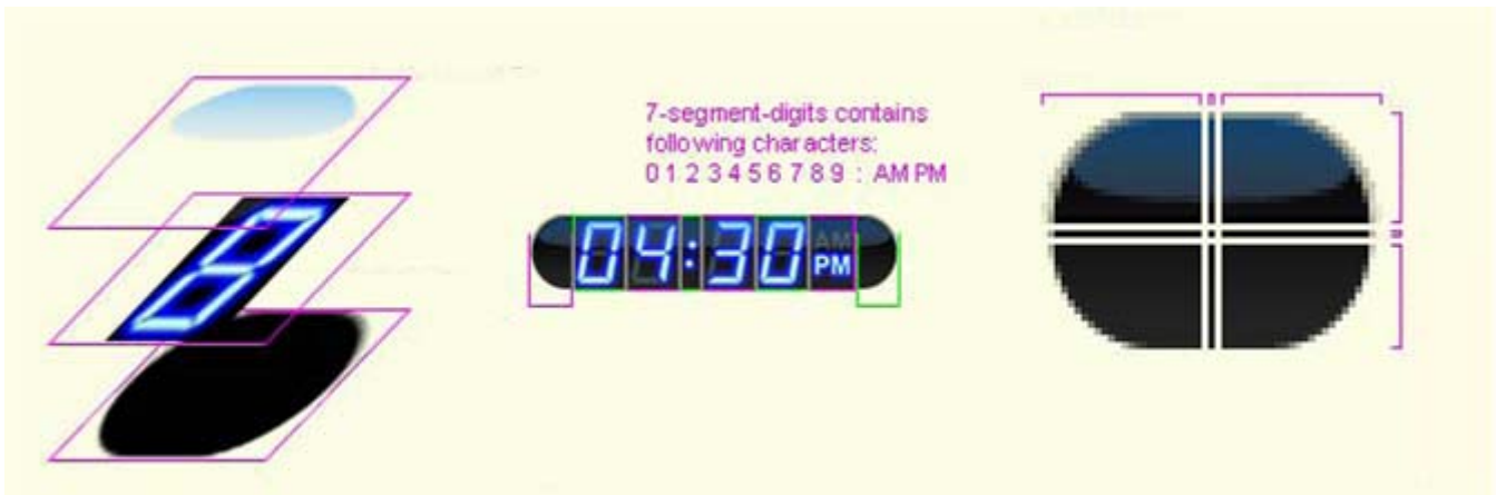
Figure 29 – The 7-segment display overlay sample
